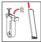
Load magazine using BB speedloader. Do not overfill magazine. (BB speed-loader included)\*
