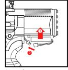
Insert battery into compartment as shown.
