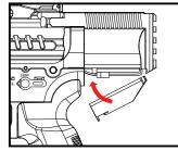
Ensure that the battery and cables are flushed flat. Close cover, making sure the tab clicks into place.
