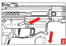
Then remove the magazine using the release button.
