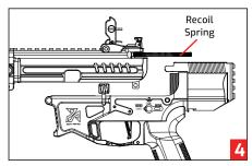
Gripping the upper receiver in one hand and lower receiver in the other, slide apart. The recoil spring will now be exposed.
