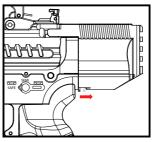
The battery compartment can be found under the picatinny stock adaptor. Pull tab back to open cover.
